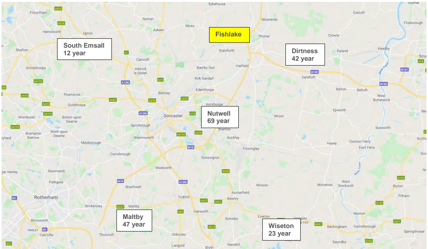
FIGURE 20: SCREENSHOT FROM GOOGLE MAPS SUMMARISING EVENT RETURN PERIOD ASSIGNMENT FROM RAIN GAUGE DATA
