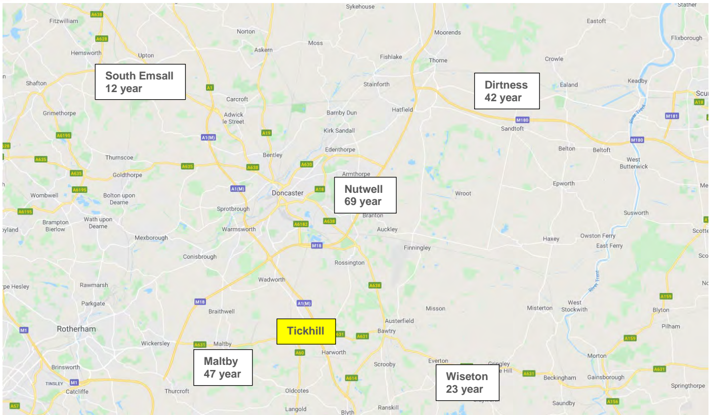
FIGURE 35: SCREENSHOT FROM GOOGLE MAPS SUMMARISING EVENT RETURN PERIOD ASSIGNMENT FROM RAIN GAUGE DATA
