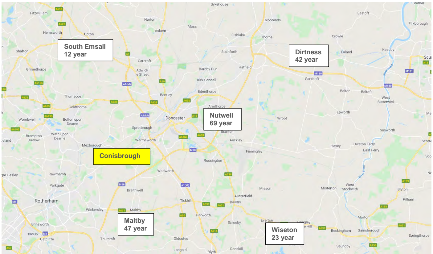
FIGURE 27: SCREENSHOT FROM GOOGLE MAPS SUMMARISING EVENT RETURN PERIOD ASSIGNMENT FROM RAIN GAUGE DATA
